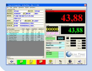
Allows the Operator to insert all the staring data (Production Order, Batch,...) and all the defects by using the precious help of the Touch Screen Technology.
